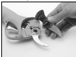
4. Remove the pin and remove the movable blade.
