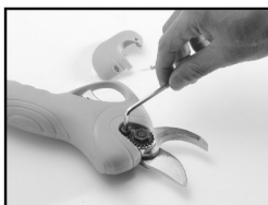
2. Remove the screws from the blade nut retaining buckle (this step is critical).
