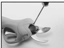
1. Remove the screws with a screwdriver and open the cover.
