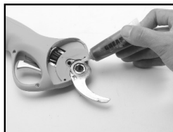
6. When replacing the blades, lubricating oil must be added between them.
